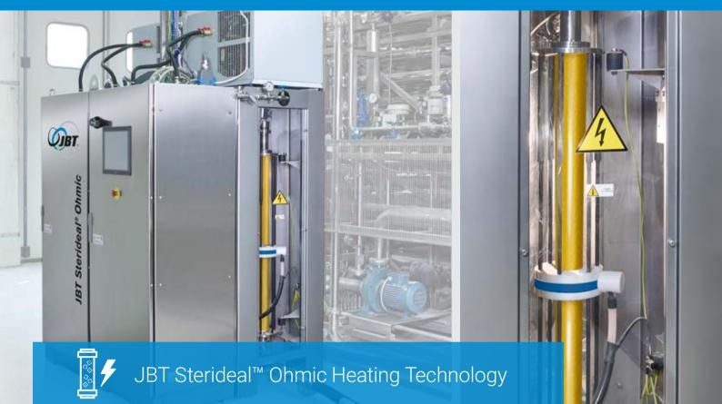
The **JBT Sterideal™ Ohmic Heater** utilizes the electrical resistance of food to generate heat quickly and efficiently. The heating speed is impressive, with a 10°C/second heating rate compared to the typical 0.5°C/second rate of conventional tube heat exchangers. This **rapid heating** results in **shorter cooking times**, preserving the organoleptic properties of food such as color, texture, and taste, while retaining nutritional value.
